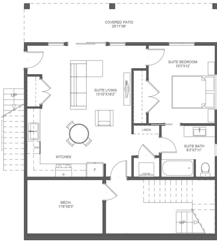
LOWER FLOOR PLAN (9' CEILING) LOWER FLOOR AREA: 247.91 Sq Ft SUITE FLOOR AREA: 631.99 Sq Ft
