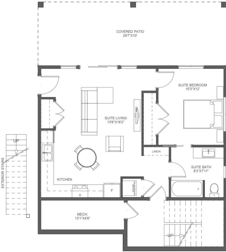
LOWER FLOOR PLAN (9' CEILING) LOWER FLOOR AREA: 191.99 Sq Ft SUITE FLOOR AREA: 611.39 Sq Ft
