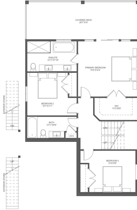
MIDDLE FLOOR PLAN (9' CEILING) MIDDLE FLOOR AREA: 980.21 Sq Ft
